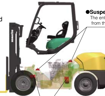
●Power train floating The engine and transmission are isolated from the frame.
