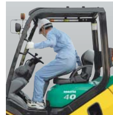
When the operator leaves the seat, OPS is activated
