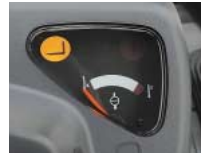
Lifting interlock lamp on the control panel
