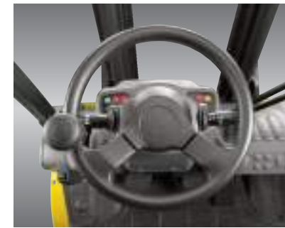
Steering wheel diameter 300mm
