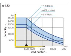
Note:Load capacity except for 500mm load center is reference only.
